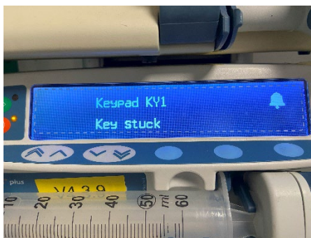
Picture 2: KY1/Stuck Key Error Displayed
