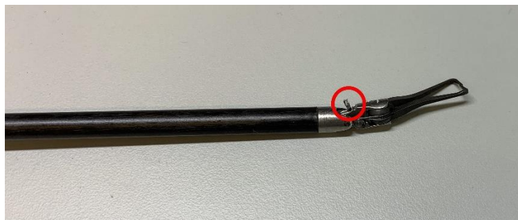
Figure F: Broken Pitch Cable
