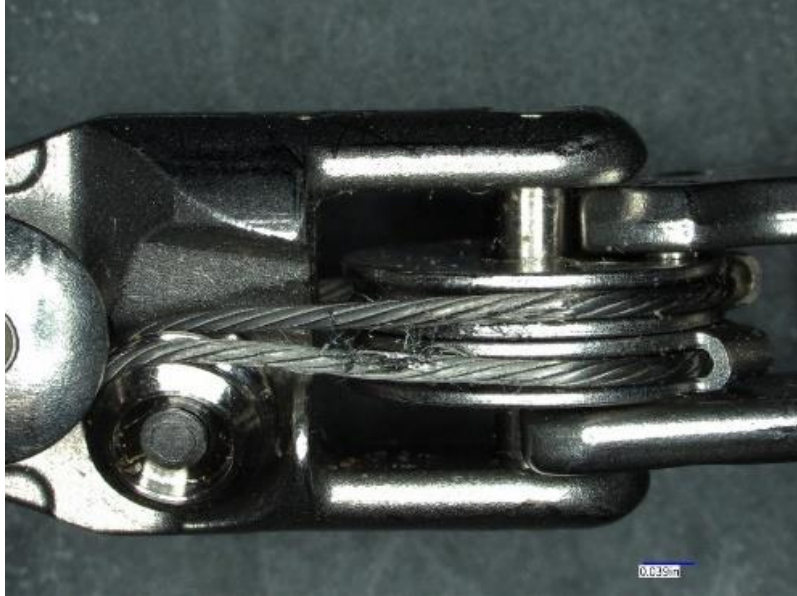
Figure D: 20x magnification of a frayed grip cable a da Vinci Xi instrument
