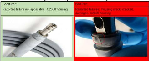
Figure 1: Example of Cracked Housing
