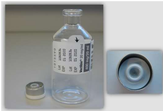
Image 2: Vial with a rubber stopper, which came off while the flip-off cap was removed
